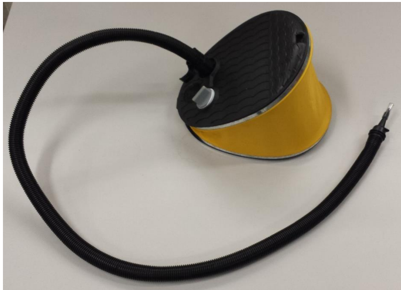
Figure 6.1. Airhead® high volume bellows pump. Shown with 3D printed piece (gray) to block flow from “deflate” port.
